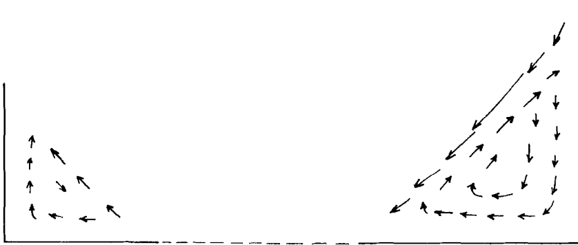
FIG. 5. "Blow-up" of corner eddies.
